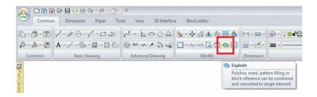
Disassemble the title block by exploding it (write explode [Enter] or click Explode button in the Modify icon group from the Common tab).
