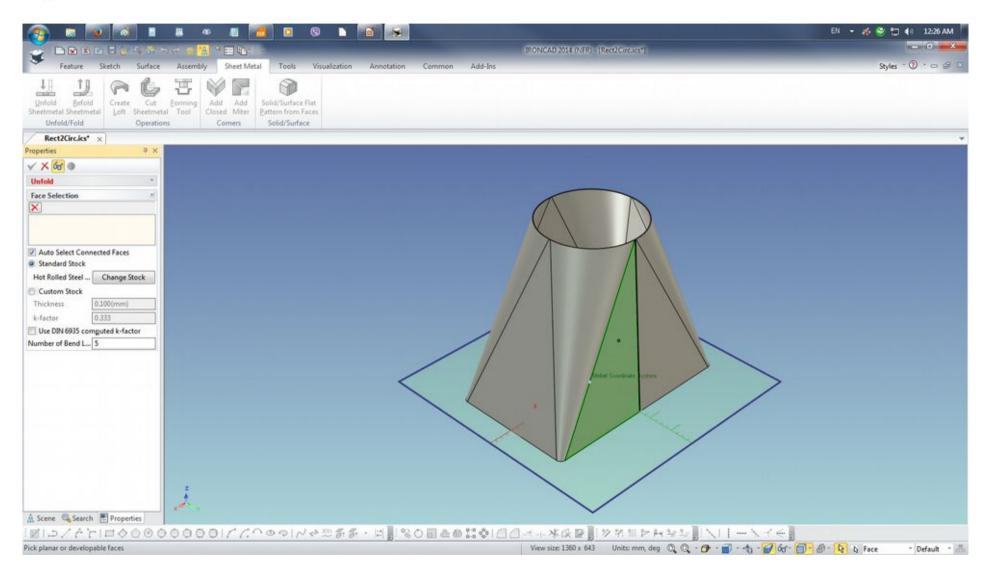
Point the cursor on the generated Part2 and perform a double LMB click to generate the bend lines. Save the file.
