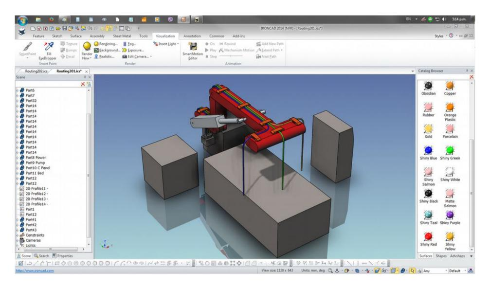
Hydraulic hose and power cables will be created using 3D Curve Tools. On the scene image, a floor slab was place as reference to the work area. On the Scene Tree, a list of 2D profile created for connection points.
