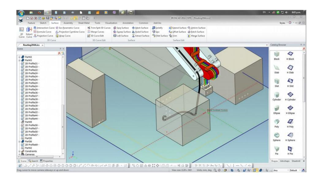
With the wiring cables Part72 created from the Part10 C Panel, the 3D Curve Tool Insert Polyline and Insert Connector will be used to connect with the other components of the machinery.
