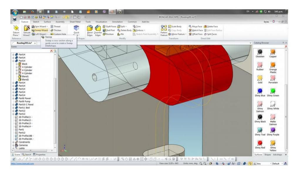
As a drawn profile was created as reference for the Sweep, this type of Create a sweep window is displayed. Note that the Create a sweep window without a profile looks different from this one.
