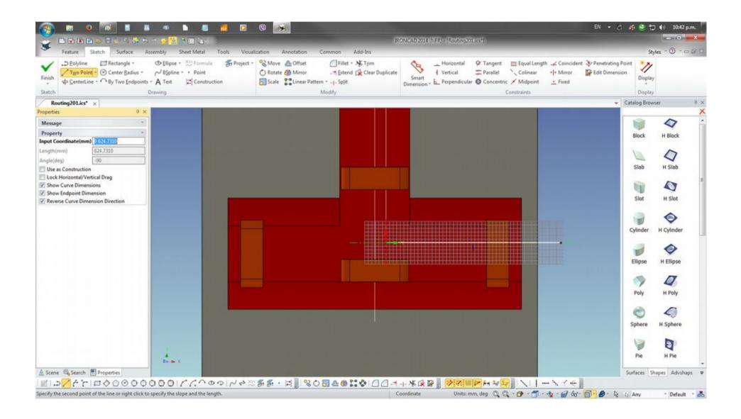
Select 2D Sketch and pick the endpoint of the line and draw a 2 point line as shown on the vertical Y axis of the drawing grid.
