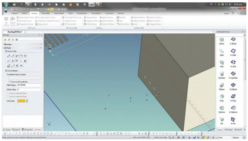
Using Insert Connector is best used for short connections. Also picking the right starting point from either object can produce better or unyielding result. This was connection was done top > down and the flow was smooth. Earlier it was drawn with bottom > up and the created corners that seem unaware of the plane it was going to. This created 3D Curve Part46
