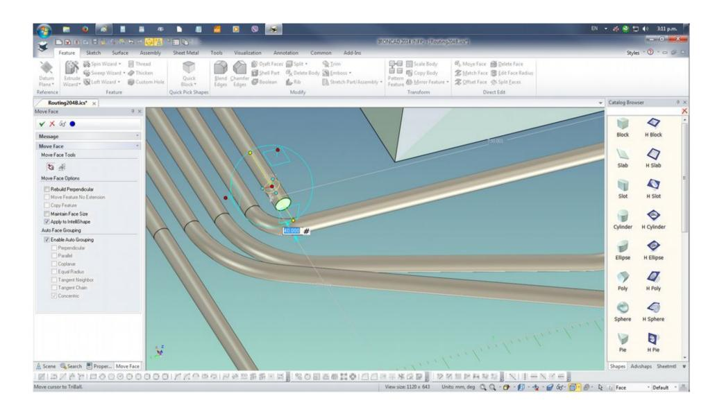
After the face has been moved, create the 3D Curve andnOn the 3D Curve Tools, select Insert Line. Depress SHIFT key before picking the center of the profile to create a perpendicular line. Insert Polyline to create the path for the connection to the pump module. Adjust the points with the TriBall to create the desired routing path. Apply the necessary fillets on the corners of the created path.
