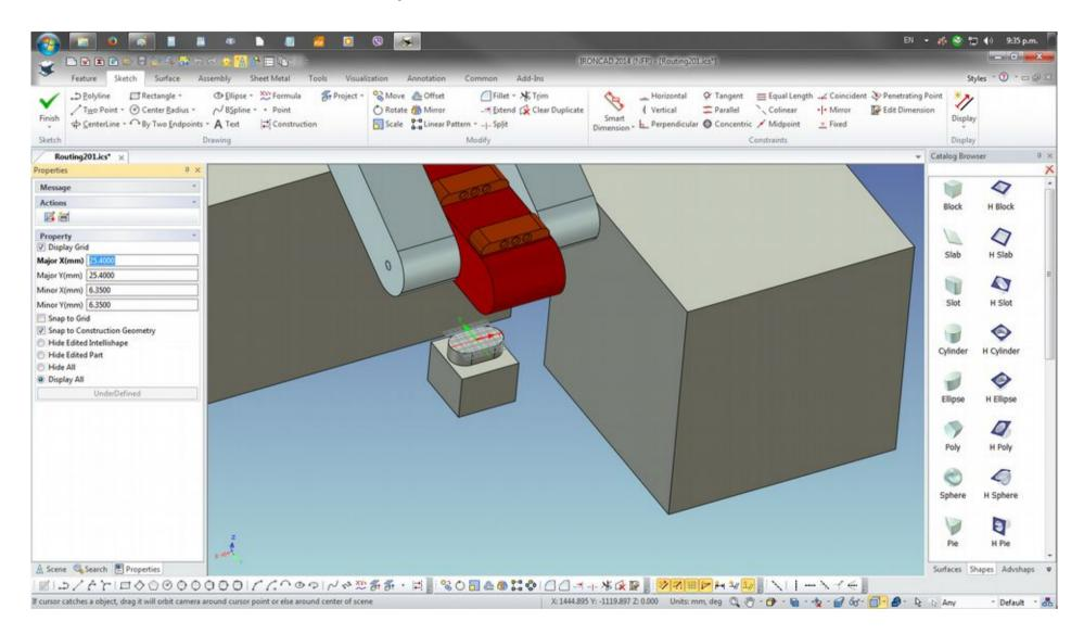
Using the F10 key to activate the TriBall, select the Y axis handle to rotate 90°
