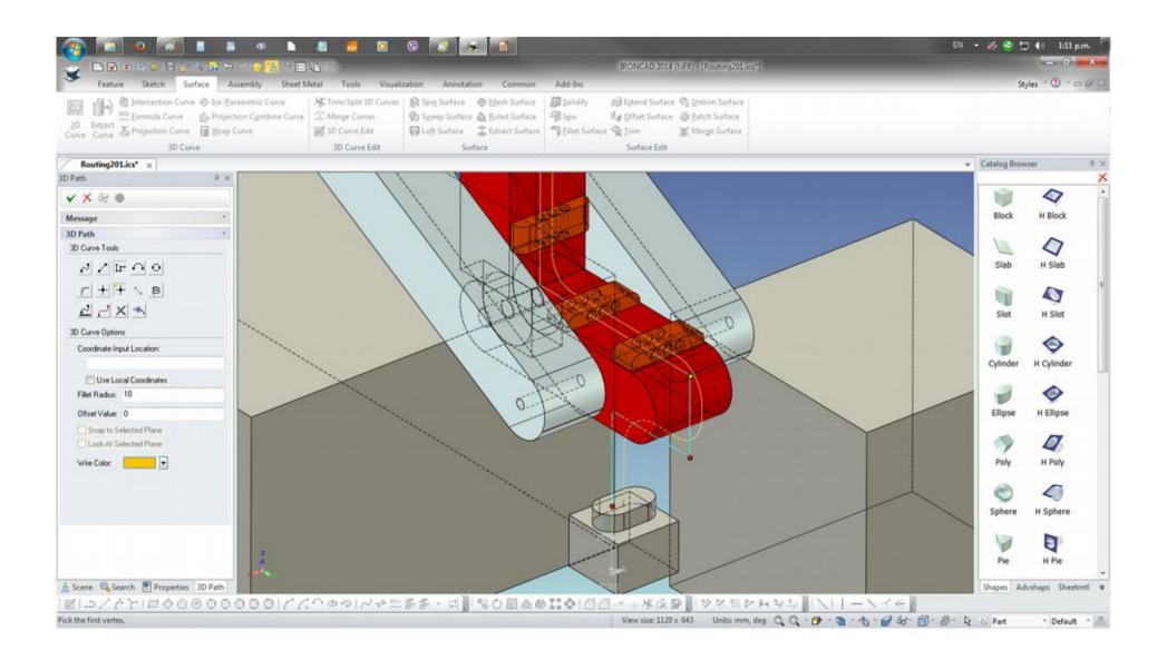
Apply the necessary fillets on the corners after creating the 3D Polyline.
