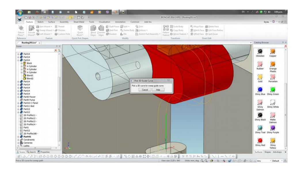
Part41 is the created Sweep from 2D Profile18A. Repeat the same process for 2D Profile 18B
