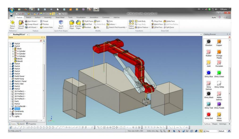
Part42 is the created sweep. The difference from Part41 is that the Sweep travels to Z, Y and X axes.
