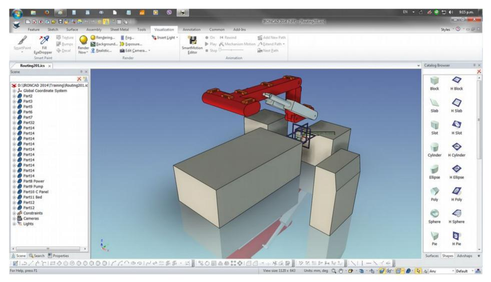
On the Scene Tree, select and suppress Part9 Pump so it will not be obstructive to the view during this part of the guide.
