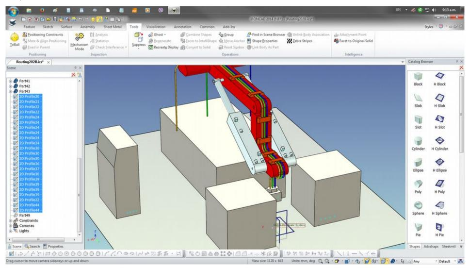
It is easier to manage making 2D Shape for the hoses from the hydraulic cylinder as it is on the Y and Z axes before it drops of the porximity of that part and connects to the pump block. A 2D Polyline Sketch and fillet was applied in this 2D scene
