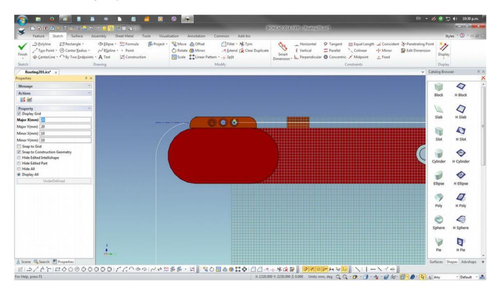
Select 2D Sketch and pick the endpoint of the line. Key F3 to Orbit or rotate the scene and activate the TriBall (F10) to orient the drawing grid flat to the surface.
