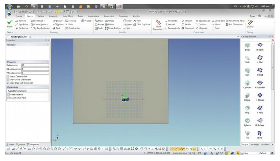
Once the 3D Curve polyline has been created, press the A key to show all planes and adjust the the size of the XY plane to guide the TriBall on that plane Alternatively, the Z key will display the XY plane only.
