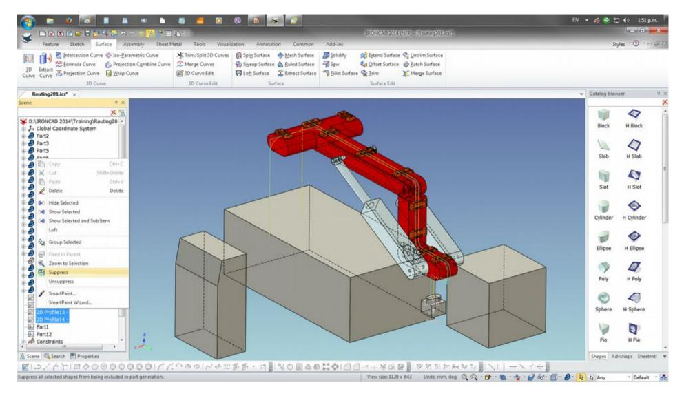
Create 2D Sketch profile for the cable to be created with Sweep. Select the center point of the diameter of the slot
