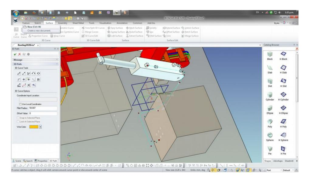
Suppress the 1<sup>st</sup> 2D Profile50 from the Scene Tree. Create a Sweep from the Feature tab and select the point and the 3D Guide Curve
