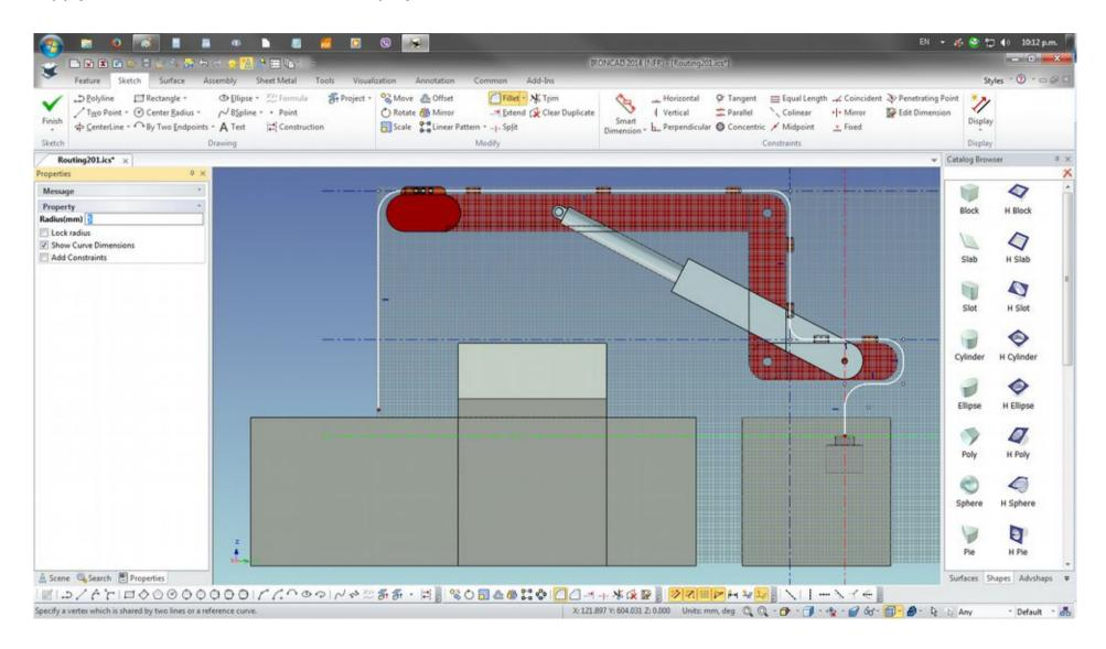
The first 2D Profile11 or Line A path. It is a 2D line path in the Y and Z axis. This Line A path will be copied to the left and edited so it goes from the Y, Z, and X axes.
