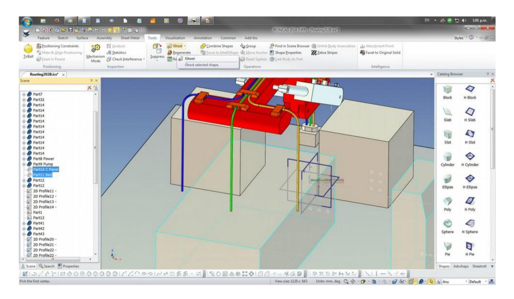
Trace the 2D Profile50 path with Insert Line, Inset Arc, Insert Polyline to create the 3D path. Using the Triball to move the points preceding the polyline after the arc onwards till the final corner to attach the end on the 2D Profile drawn on the Part9 Pump. This created 3D Curve Part30
