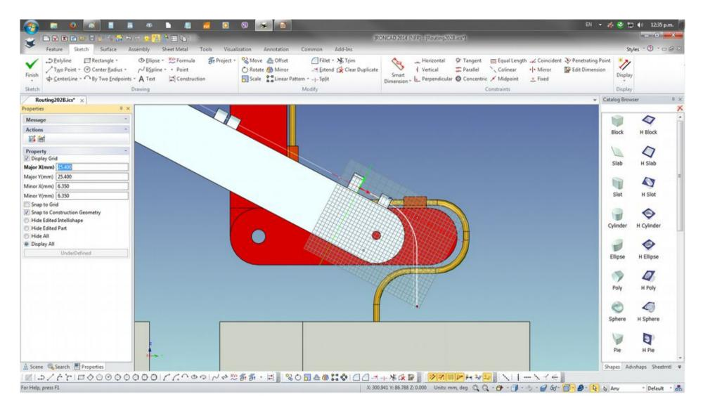
Copy and position the created 2D Profile 50 and 57 accordingly. Notice that the Position Dimensions is activate on the scene it can precisely placed
