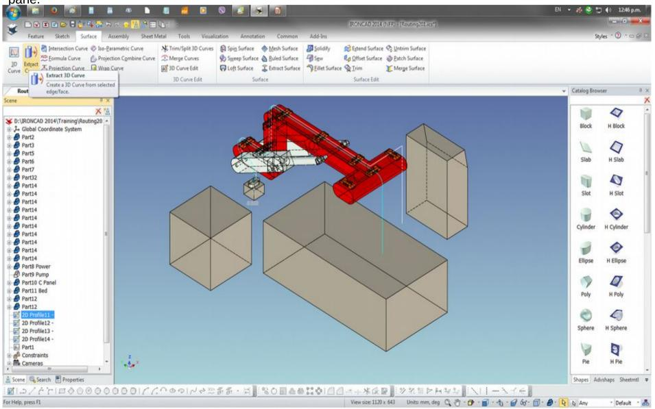
Again, I've used F3 to Orbit/orient the scene. I have edited 2D Profile12 to remove fillets so it easier to use as a guide for creating a new 3D Curve.
