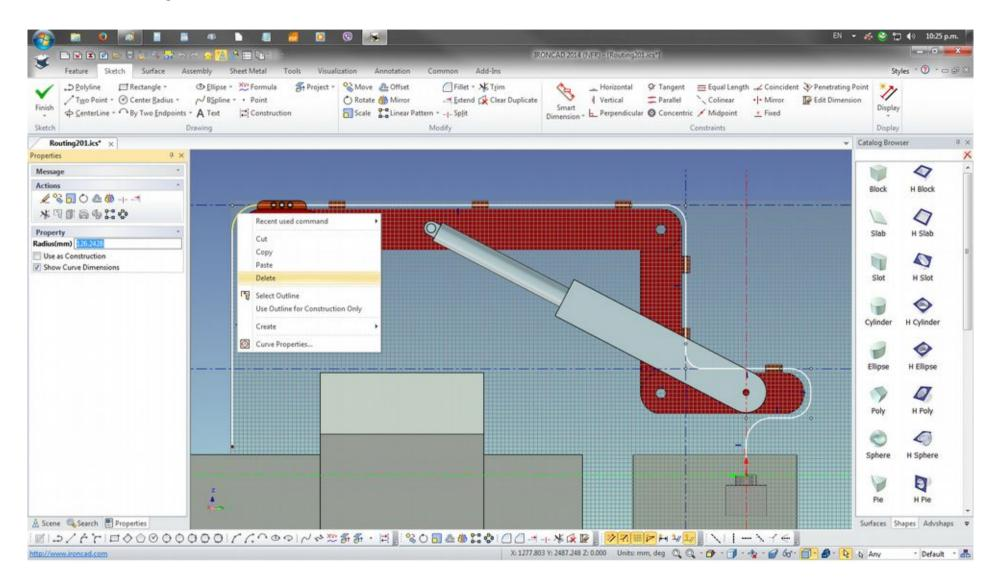
Move the remaining endpoint to the center of the third cable block hole.
