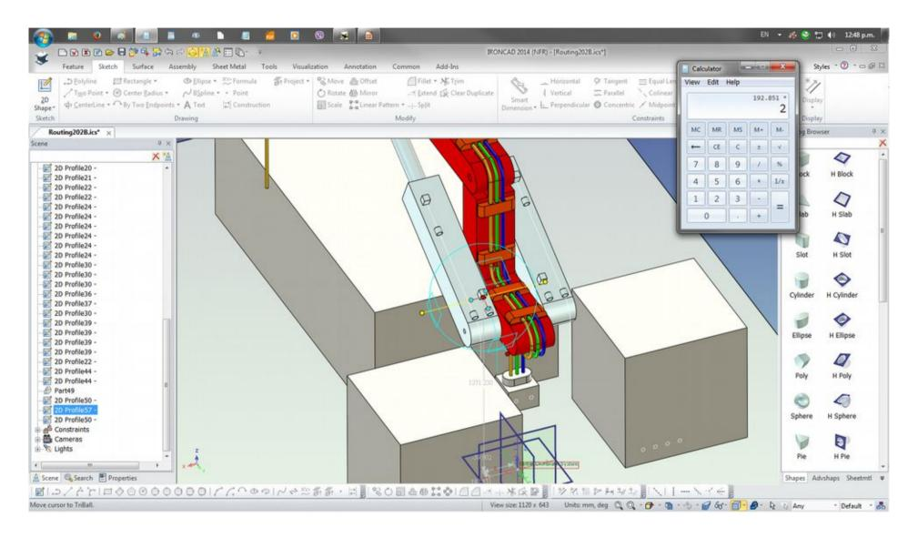
Select Part10 C Panel and Part11 Bed and apply the Ghost feature from the Tools tab so it is easier to use the 3D Curve Tools to create the 3D path connections
