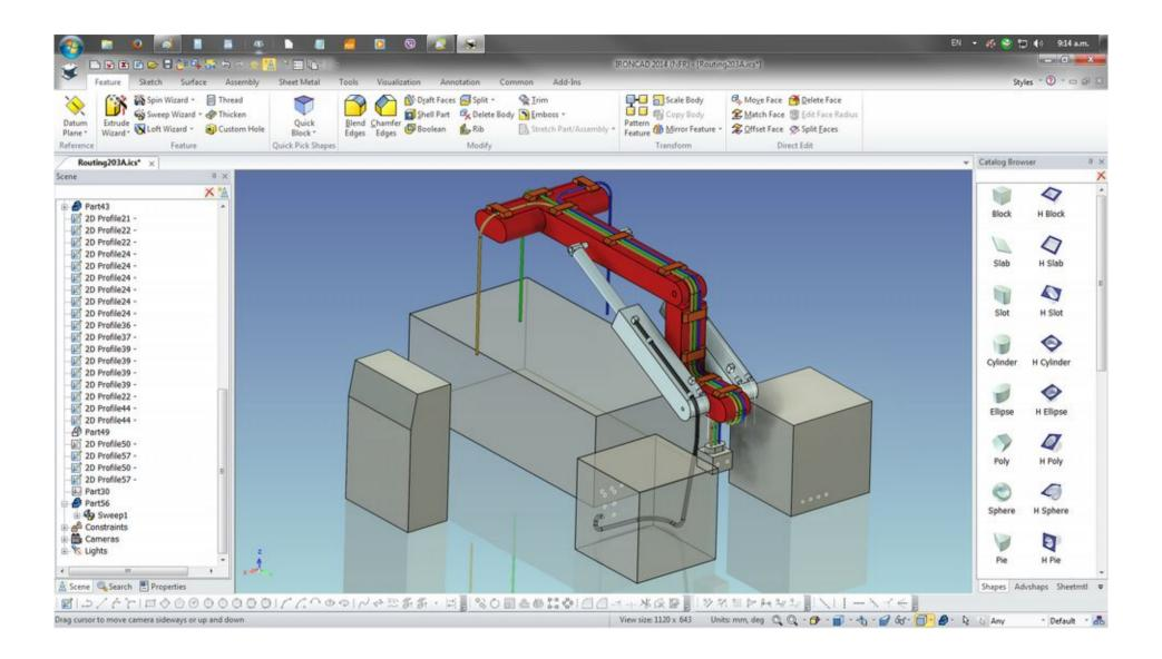
After drawing a 2D sketch reference 20 mm Ø of a power point, select Move from the Actions dialogue panel.
