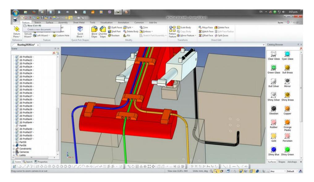
Create 3D Curve wiring using the Insert Connector tool. Note that using the Insert Connector Tool can produce different paths depending on the features used. First screen shows the Planar Connector Options set by the program.
