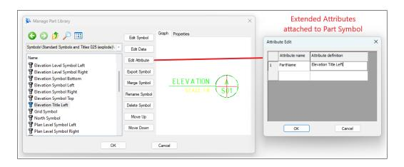
For consistency, the names used for System and Custom Part Properties within the 3D Scene, should be used for Attributes and Extended Attributes of Blocks as well (if applicable). These need to be listed within the "Set Matching Rule" (within Options).
