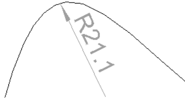
Figure 3-37 Curvature radius dimension - example
